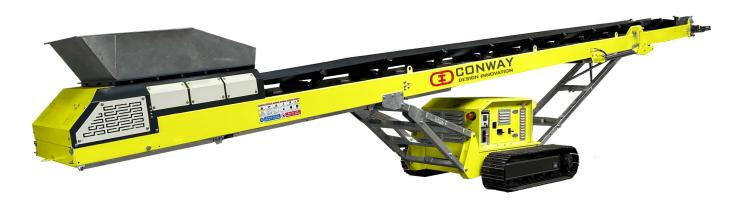
CDI offer the TRACKED CONVEYOR range of self-powered medium-duty track mounted conveyors with a range of options. The simple yet robust design provides an effective solution to fit many producers need for a medium capacity tracked stockpile. These conveyors offer real value for money and can be containerised for cost effective shipping worldwide. Now available in Both Diesel/Hydraulic and Dual Power Electric/Hydraulic for maximum efficiency and Minimum Running Costs.
